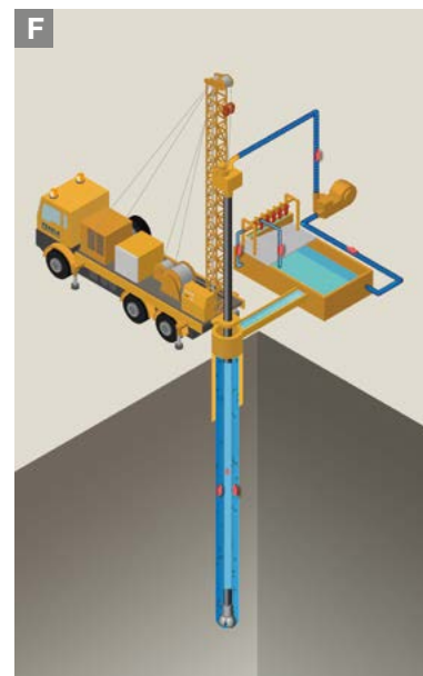
D Im-Loch Hammer Bohren Down-the-hole hammer drilling (DC)
